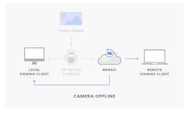
When the camera is offline, or the timestamp for the video file exceeds the camera's hardware memory capacity, all video will be viewed as a remote stream, with viewing devices retrieving video data from the cloud.
