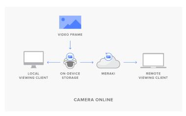
When cloud archive is enabled on a camera, and the camera is online, data flow will follow the standard path: both local and remote viewing devices will pull video directly from the camera memory. A backup video file is stored in the cloud, but not utilized in this case.
