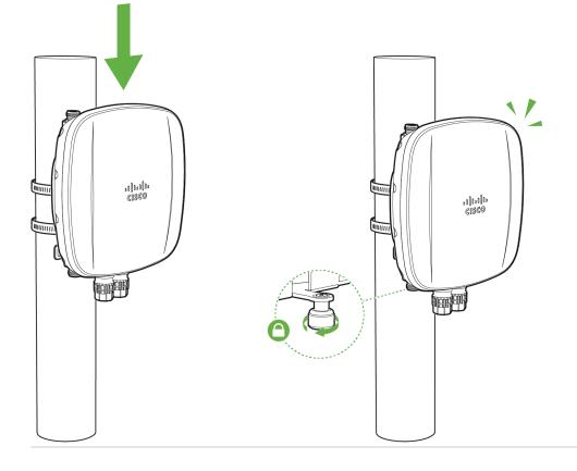
4. Slide the mounting slots on the back of the AP over the mounting posts on the mounting plate. The AP is securely attached when an audible click is heard.
