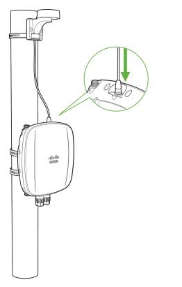
4. Remove the protective cap and connect the antenna to the GPS port on top of the CW9163E.
