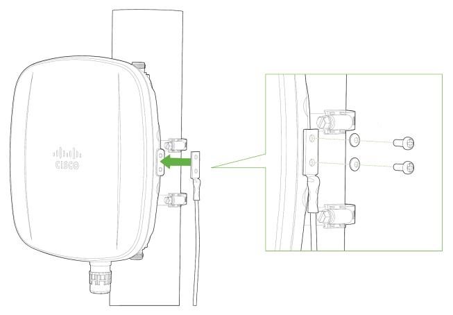
3. Connect one end of the grounding strap to the grounding post with included screw and washer. Securely attach the other end to a nearby metal structure.
