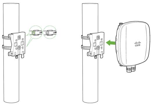
3. Secure the mounting bracket by tightening the screws of the mounting straps. To tighten, use a flathead screwdriver.
