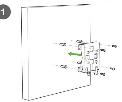
1. To mount the AP on the wall, use the mounting bracket as a template to mark the locations of the mounting holes on the bracket.
