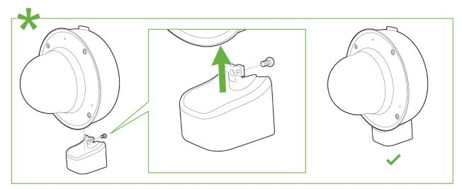
4. MV13 series comes with two base mount plates, a small plate and a large plate. The functionality of both plates is identical. Please refer to the guidelines below on using the base plate mounting to any surface or on top of a mounting accessory.
