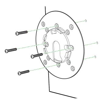
Installing the conduit box to MV13 series: (optional)
