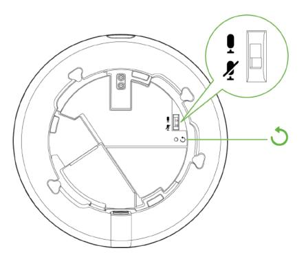
The MV13 also features a Factory Reset button which lies right under the microphone cut-off switch. This reset function can be activated by inserting a reset pin into this section for 15 seconds. Do not that this action deletes all the data in the camera including the stored video, and it is not reversible.
