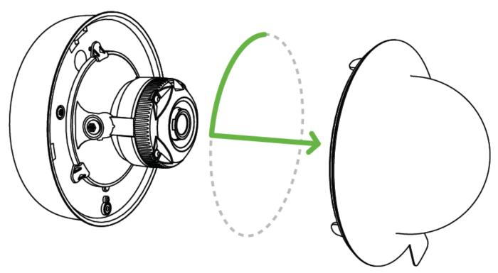
5. Align camera to mounting plate studs. Slide the camera onto studs and turn the camera clockwise to secure the top plate. If the cable run is not coming directly behind the camera, the cable guard will need to be removed. Below are two mounting examples.
