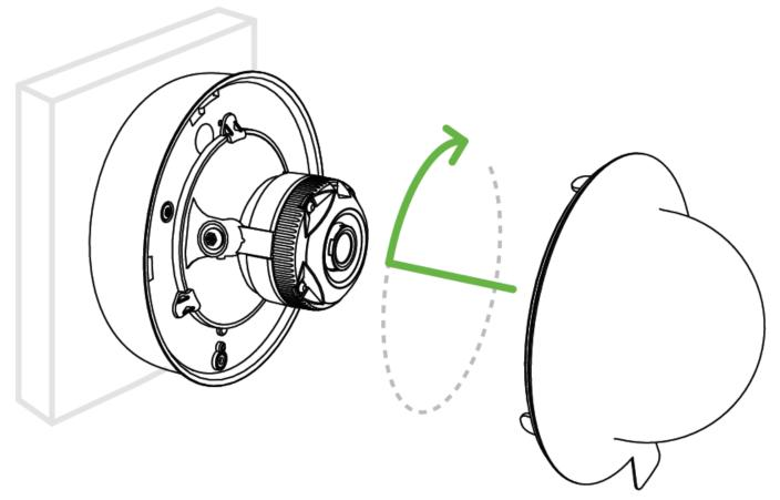
9. Remove the protective cap from the camera bubble.
