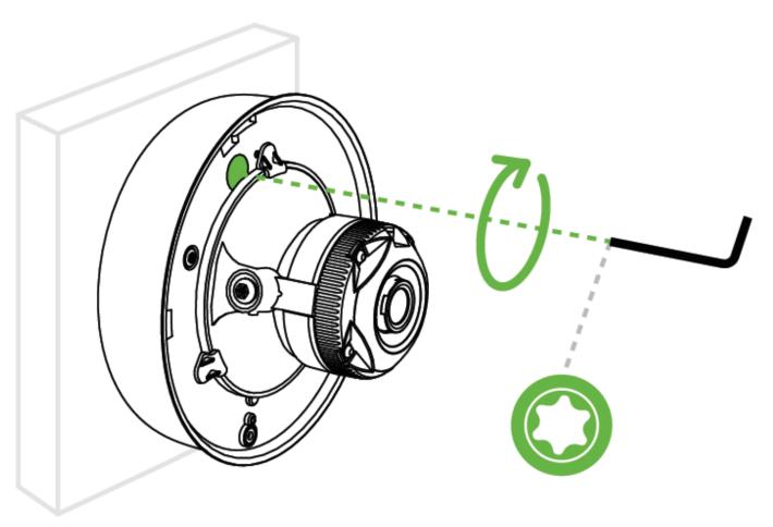
7. Aim the lens. Inspect the camera feed on the Meraki Dashboard to fine-tune the picture. The camera sensor and lens unit can be physically tilted through a range of 65 degrees, rotated through a range of 350 degrees, and panned through a range of 350 degrees. The image can only be rotated by 180 degrees in software, and no other adjustments can be made. Zoom and focus can not be adjusted on the camera.
