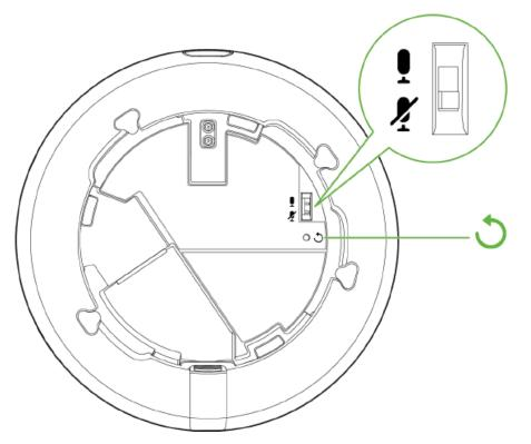
The MV33 also features a Factory Reset button which lies right under the microphone cut-off switch. This reset function can be activated by inserting a reset pin into this section for 15 seconds. Do not that this action deletes all the data in the camera including the stored video, and it is not reversible.
