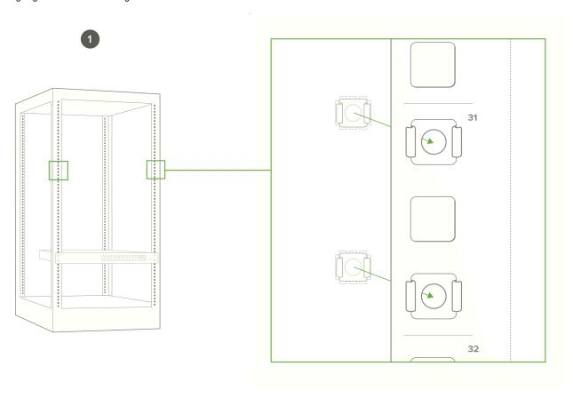
2. Attach the switch face plate to the cage nuts on the rack.
